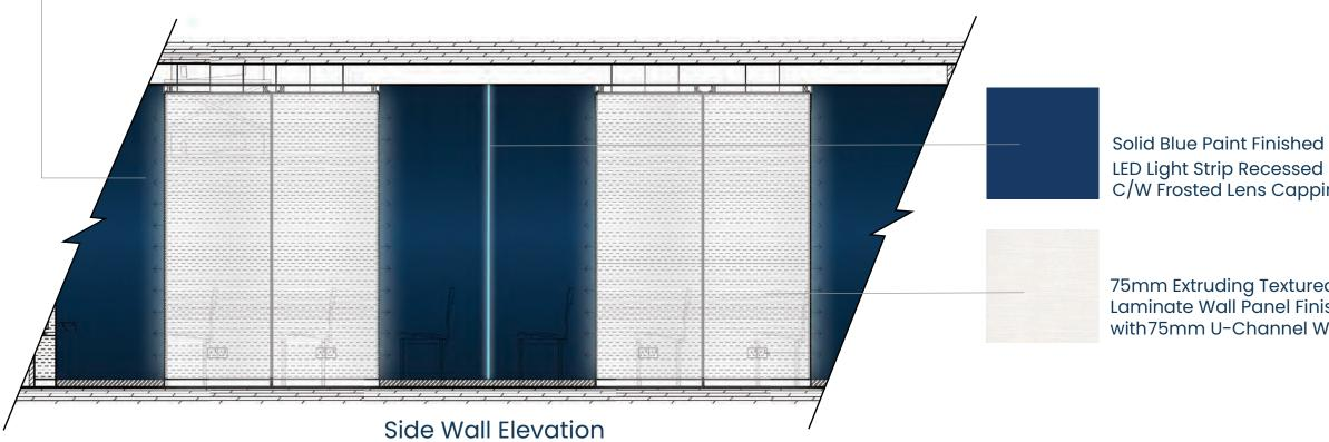
LED Light Strip Recessed Lighting C/W Frosted Lens Capping.
