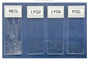
Methodology: **Soap scum** glass slides were rinsed with a 1 M calcium oleate solution for 3 min then dried for 2 h at 70°C (3 cycles) and dipped in a shower cleaner for 2 min. **Limescale** glass slides were rinsed with a 2 M calcium carbonate solution for 3 min, then dried for 2 h at 70°C (3 cycles), then dipped in a shower cleaner for 2 min. **Formula containing**: NEG: No polymer at pH 7, LYG 2: 1% Soltellus at pH 7, LYG 5: 1.5% Soltellus at pH 9, POS: Leading brand.
