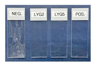
Methodology. Soap Scum Glass slides were rinsed with a 1 M calcium oleate solution for 3 min then dried for 2 h at 70°C (3 cycles) and dipped in a shower cleaner for 2 min. Limescale Glass slides were rinsed with a 2 M calcium carbonate solution for 3 min, then dried for 2 h at 70°C (3 cycles), then dipped in a shower cleaner for 2 min. Formula containing: NEG: No polymer at pH 7, LYG 2: 1% Soltellus at pH 7, LYG 5: 1.5% Soltellus at pH 9, POS: Leading brand.
