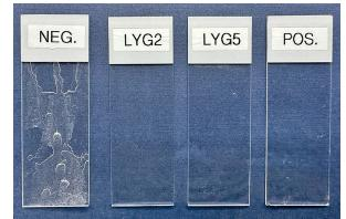
Methodology: **Soap scum** glass slides were rinsed with a 1 M calcium oleate solution for 3 min then dried for 2 h at 70°C (3 cycles) and dipped in a shower cleaner for 2 min. **Limescale** glass slides were rinsed with a 2 M calcium carbonate solution for 3 min, then dried for 2 h at 70°C (3 cycles), then dipped in a shower cleaner for 2 min. **Formula containing**: NEG: No polymer at pH 7, LYG 2: 1% Soltellus at pH 7, LYG 5: 1.5% Soltellus at pH 9, POS: Leading brand.
