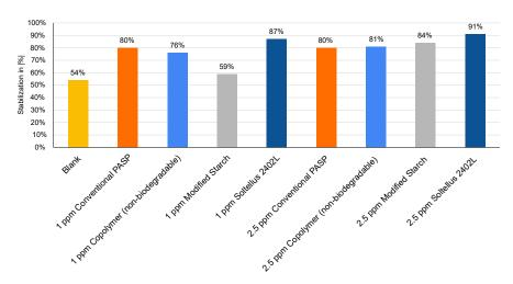
Third-party Once-Through DMEG tests were conducted with Soltellus and conventional scale inhibitors at a low dosage of 2 ppm. Soltellus inhibited scale significantly longer than conventional PASP and non-biodegradable alternatives. The method involved calcium and carbonate solutions pumped through a heated capillary, measuring pressure increases over time.
