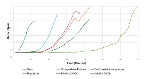
Third-party Shaker Bath tests were conducted with Soltellus and other conventional scale inhibition alternatives at low dosages of 0.5 ppm, 1.0 ppm, and 2.5 ppm. Soltellus showed better calcium carbonate stabilization than current conventional polyaspartate (PASP) offerings and performed on par with conventional non-biodegradable alternatives.
