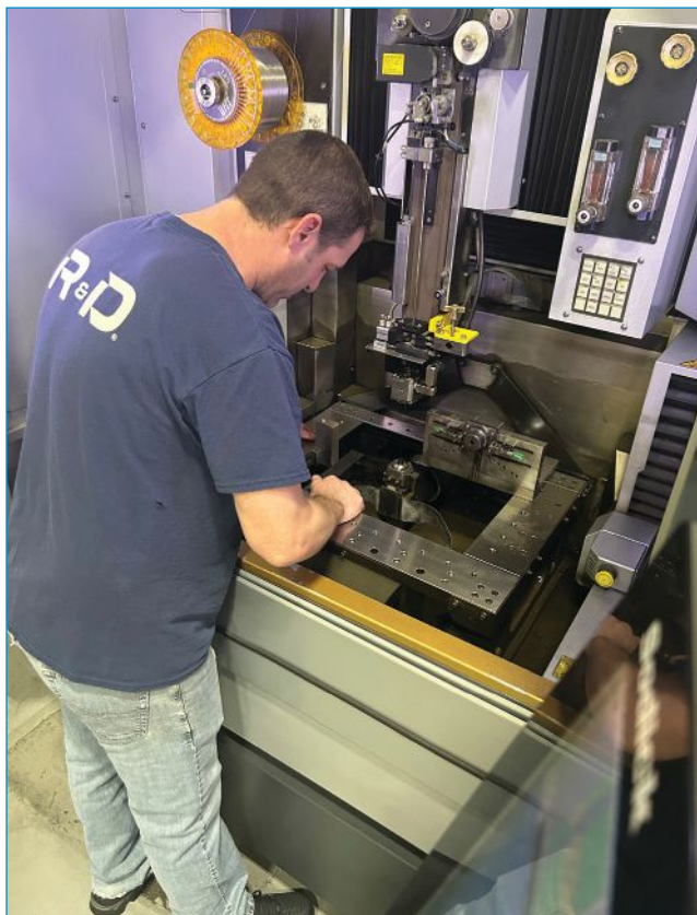
The team uses ultra-precision wire EDM technology for advanced machining applications.
