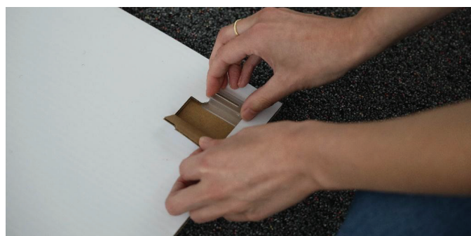
2: Slide plastic joiners onto each of the eight slots on the outer curved edges (flip the cardboard flap out to place the joiners in and fold it back over to secure).
