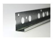
Stucco Stop is made from .018" thick galvanized G90 steel and is used to provide a quality, finished edge for stucco.
