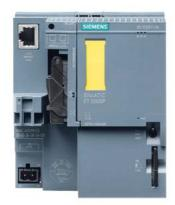
\*\*\* spare part \*\*\* SIMATIC DP, CPU 1512SP F-1 PN for ET 200SP, central processing unit with work memory 300 KB for program and 1 MB for data, 1st interface: PROFINET IRT with 3-port switch, 48 ns bit performance, SIMATIC Memory Card required, BusAdapter required for port 1 and 2
