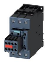
power contactor, AC-3e/AC-3, 65 A, 30 kW / 400 V, 3-pole, 24 V DC, 0.8-1.2\* Uc, with integrated varistor, auxiliary contacts: 2 NO + 2 NC, screw terminal, frame size: S2, captive auxiliary switch, suitable for PLC outputs
