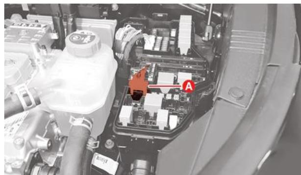
※ *The high voltage service interlock connector cannot be completely removed.*
