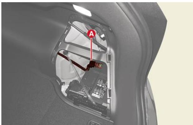
d) Disconnect the service interlock connector
