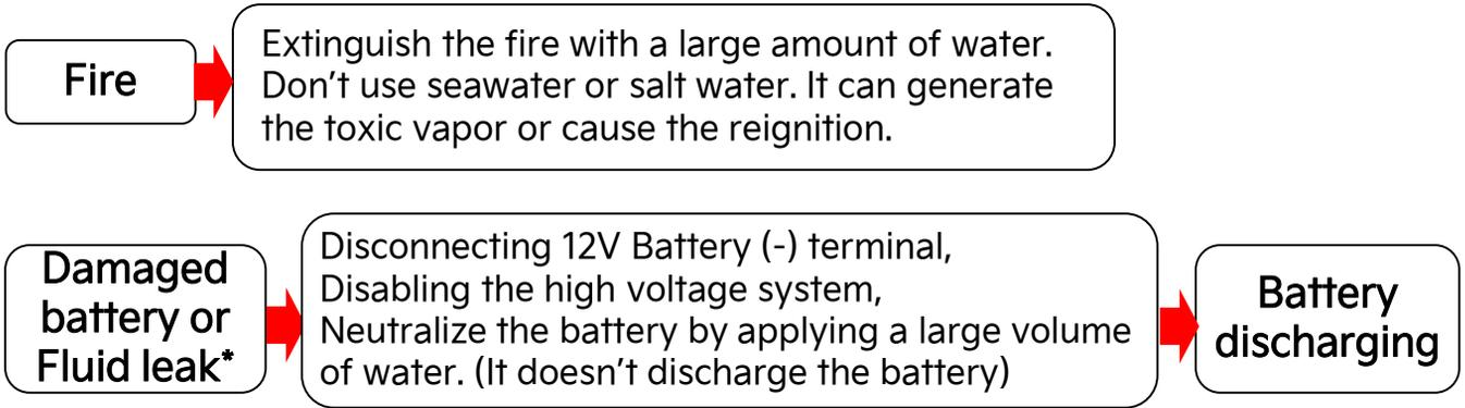
\*If electrolyte solution leakage, or any damage to the H.V battery casing is observed
